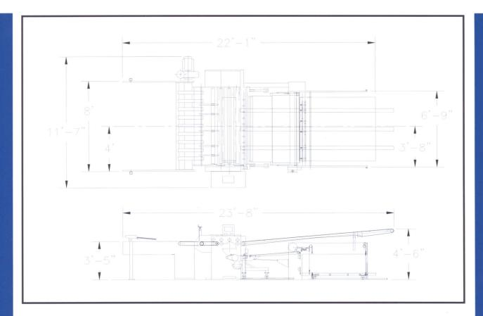
Model EM Litho Labeler with automatic board and label feeders.
